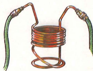
(Left): The counter-flow chiller runs hot wort through a tube that is within a tube of cold flowing water.
